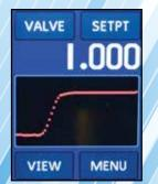
A graphical mode displays real time flow.
