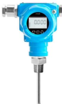
KC-8200 integrated temperature transmitter adopts ASIC&SMT signal transmitting module, optional built-in backlight and button operation LCD display module. The integrated transient voltage terminal satisfy 4 grade standard (difference-mode voltage 2000V, common-mode voltage 4000V), suitable for bad surge voltage occasions. This integrated temperature transmitter provides a flexible and reliable solution for any temperature measurement applications.
